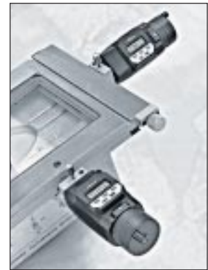
Typical application on Toolmaker's microscope.
