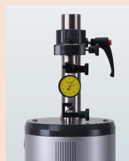
Using dial test indicator attachment set (02ASK000)
